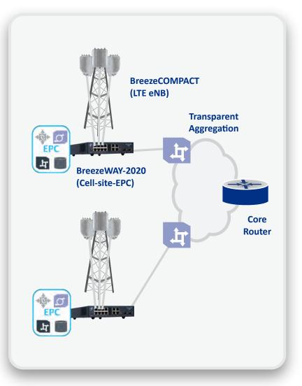
• BreezeWAY-2020 local aggregation EPC – the difference between the cell-site and this topology is that, in this case, the BreezeWAY-2020 uses its scalability to locally aggregate a few cell-sites. In this cell-site topology, more efficient localized mobility is possible, adding great value.
