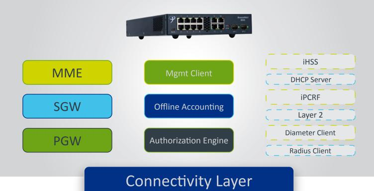
As per the illustration above, Telrad's EPC's architecture fundamentals create the most optimized, scalable LTE core solution for BWA networks enabling a combination of fixed and mobile services.
