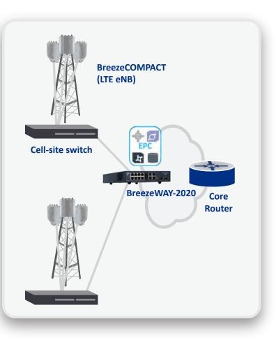
BreezeWAY-2020 Central EPC – the BreezeWAY-2020 distributed architecture is a very advanced solution for Centralized EPC compared to any EPC solution currently on the market. BreezeWAY-2020 EPC supports advanced capabilities of load balancing, m+n redundancy and
