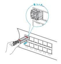
**NOTE:** Line up the module with the port and slide it gently into the port until the lock is fully seated.
