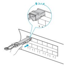
**NOTE:** When inserting a QSFP+ module, the label needs to face down.
