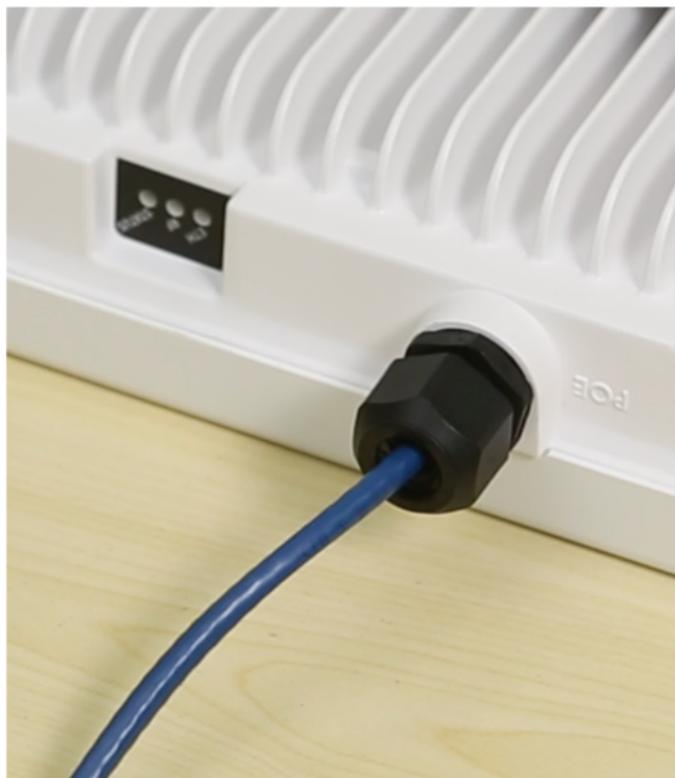
Properly terminate and test the Ethernet cable run before proceeding. This should include power verification on all pins of the Ethernet cable using a PoE tester.
