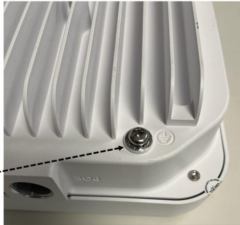
**Step 2.** Torque the screw to 6 N-m (4.5 lb-ft). The grounding wire should not limit the adjustment of the antenna.
