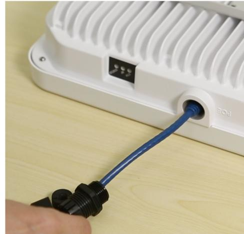
**Step 5.** Insert the cable into the RN Ethernet port and screw the cord grip body into the RN, taking care to not cross thread the plastic threads of the cord grip body with the aluminum threads of the RN enclosure.
